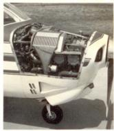
mized. The exhaust system has been designed to match exhaust gas paths to the turbo inlet from the left and right-hand cylinder banks.
